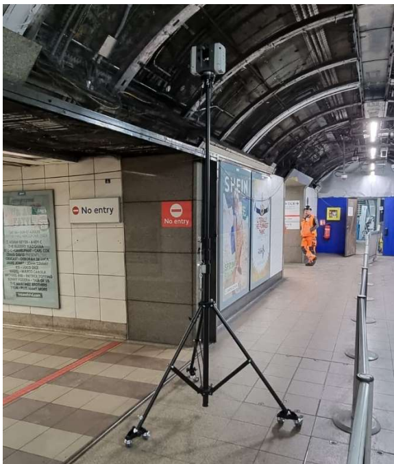
Scanner being used at Bank Underground Station for surveys ahead of undergoing drawings.
